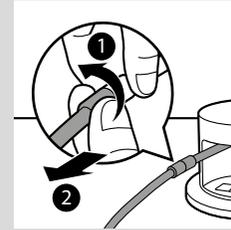
4. Use both hands to disconnect the connector. Hold one side of the connector with one hand and use two fingers of your other hand to turn the connector. Make sure you hold the plastic part and not the hose.
